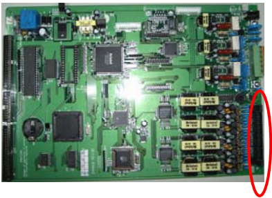
Figure 11: CO line installation
