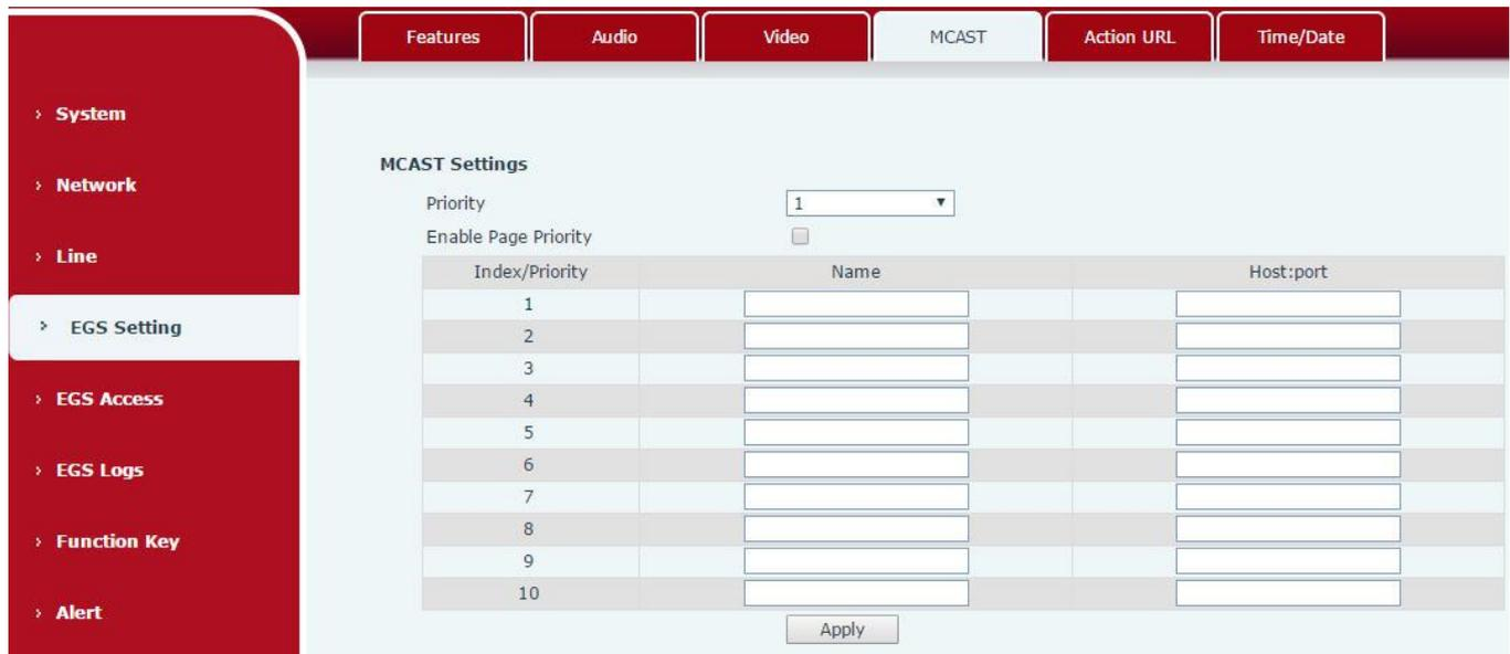
It is easy and convenient to use multicast function to send notice to each member of the multicast via setting the multicast key on the device and sending multicast RTP stream to pre-configured multicast address. By configuring monitoring multicast address on the device, monitor and play the RTP stream which sent by the multicast address.
